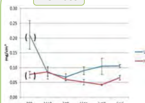
Fig. 3 AFDM measurements of biofilms developed in urban and hospital treated effluents
